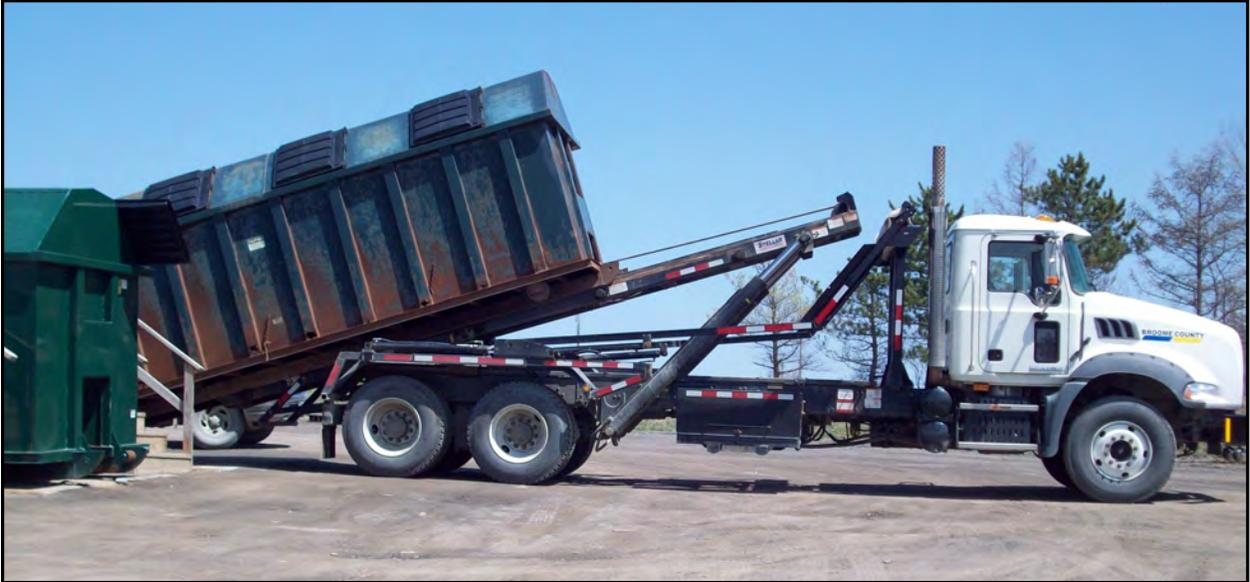
Photo 4: Pulling Recycling Roll-off
