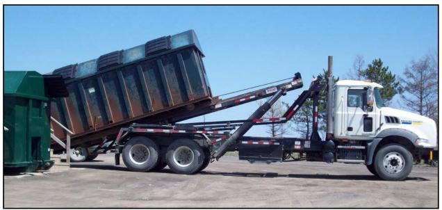
Photo 4: Pulling Recycling Roll-off
