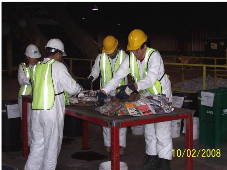
Figure 1-1. Sorting Recyclable Materials Into Various Categories.
