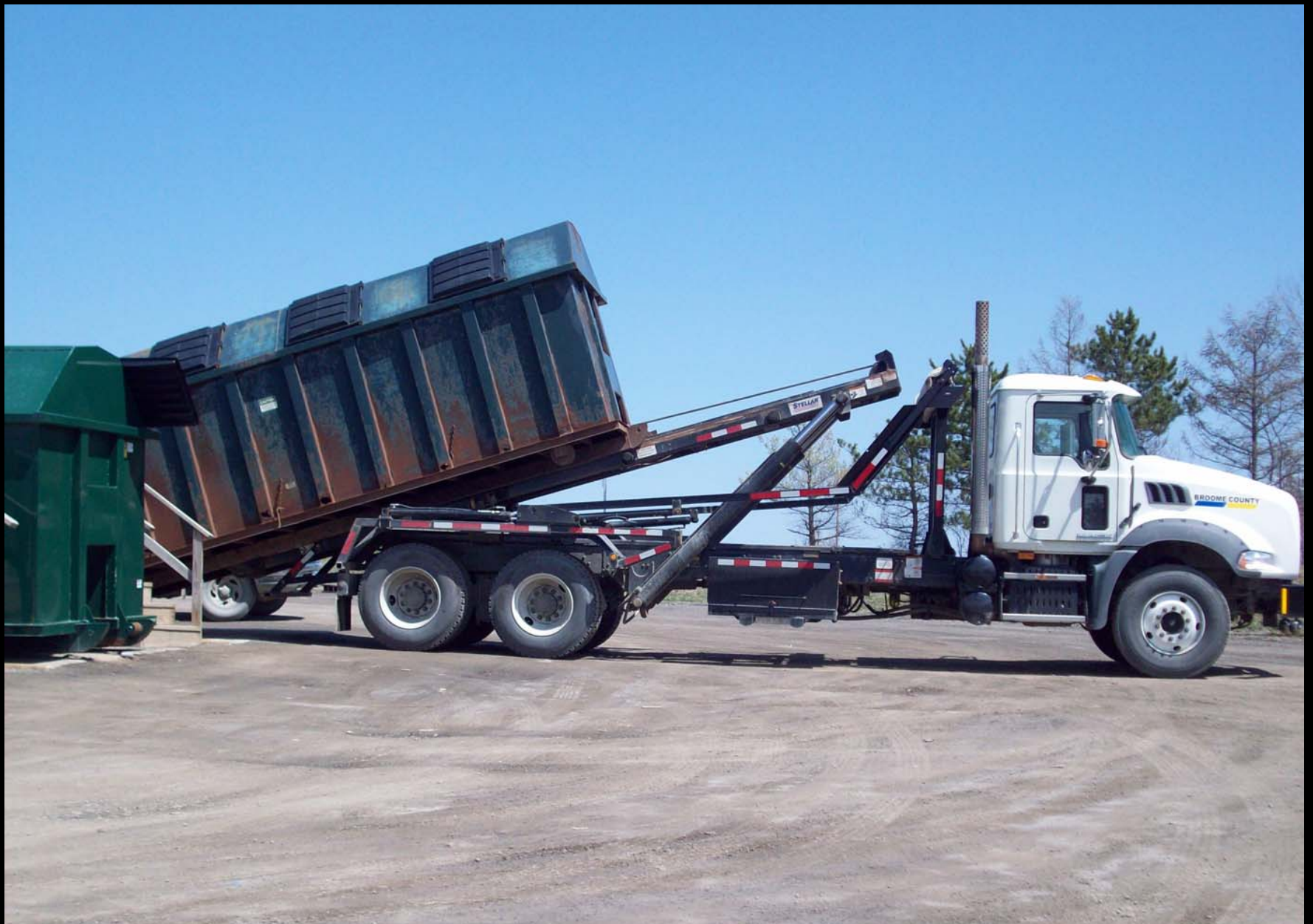
The roll-off truck pulls the container onto the bed of the truck.
